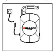
Note: The control box is water resistant, but not water proof, due to the cooling vents on the back. It is your responsibility to protect the control box from water damage, as water damage to the control box is not covered under the manufacturers warranty.
