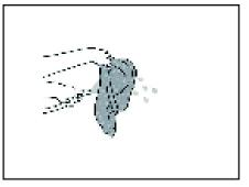
At the end of the cleaning cycle, place the robot on the caddy, disconnect the floating cable from the control box, wind the floating cable in a circle by hand and place it on the caddy hanging bracket.
