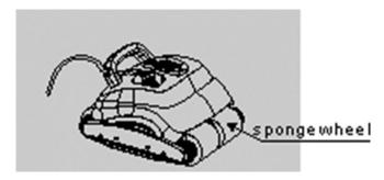
• The sponge wheels play an integral role in the balance, and cleaning effectiveness of the robot. They may take up to 1 hour to fully saturated. Please keep the robot on the FLOOR ONLY MODE (Climb/Power light showing Blue) for the initial 1 hour cycle.
